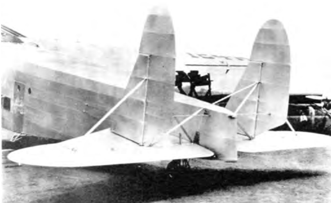
Empennage details of the first Fokker F-32 that show its two tail configuration. (Fokker via James J. Sloan)
