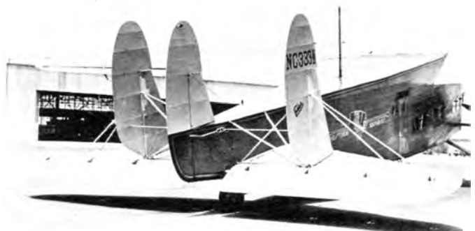
Three tail configuration used on all but the first F-32 as seen on the third plane. (Western via Bob Hufford)
